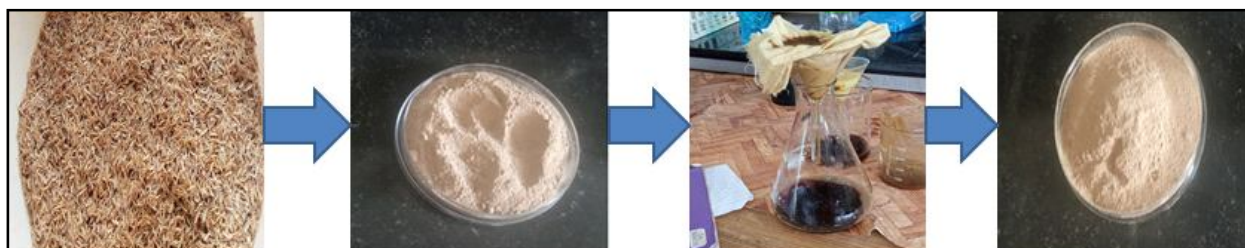
Fig. 1. Preparation of rice husk biosorbent in dye removal process.
